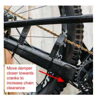
Note: Take care when trimming the STFU damper modules, we have been able to join cut segments together using additional cable ties when we have cut them too short but this is not an ideal solution.
