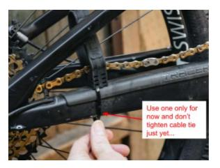
8. Shift your bike through your entire range of gears taking note of the top and bottom most gears. Modify the position of the STFU so the chain does not rub on the STFU in any position. Having a bike stand or partner for this will make the job a lot easier.
