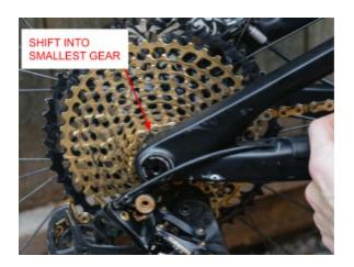
3. At the point marked in Step 1 - measure from the top surface of your chain stay to the bottom of your chain, directly above this point.
