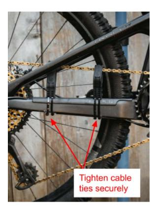
11. Trim the excess off the cable ties and double check alignment by shifting your bike through the full range of gears and inspect everything is still positioned as it should be.
