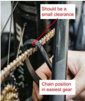
9. If the chain is rubbing in top gear (smallest cog or hardest gear) and sliding the STFU towards the cranks (10 mm or so) doesn't fix this then trimming the height of the STFU by 5mm may be required. Before
